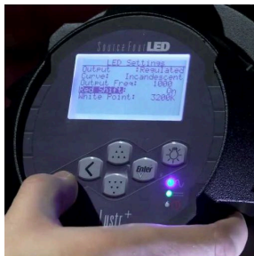
Source Four Lustr2 luminaire Control Interface and Processor
